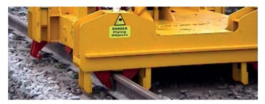
he Thomson Mk3 Fastclip attachment is the industry standard machine in the UK.
