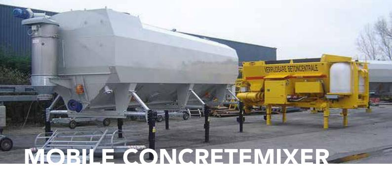
The mobile concrete mixer is the optimum machine for construction sites where concrete must be produced on site. With the mobile concrete mixing installation you can produce concrete in a precise, sustainable and individual way.
