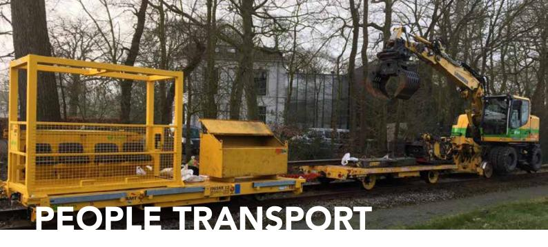
Approved safe passenger transport frames, to be mounted transversely or in the longitudinal direction so that there is sufficient load space.
