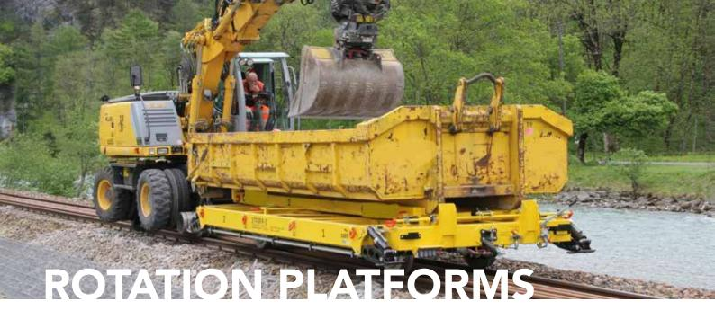
Turntables based on the ACTS-VDL system. Integrated in the trailer or with twist lock.
